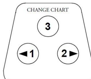
**Figure 4.** Pressure Sensitive Chart Buttons
