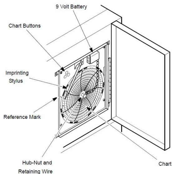
**Figure 3.** Six Inch Chart Recorder
